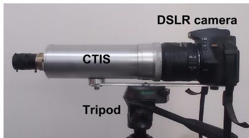
Fig. 5. Implementation of the CTIS system.
